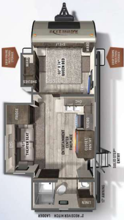
2511S REAR LIVING MINI LITE UWW: 5492 HITCH: 714 AXLE: 4719 CCC: 1382 LENGTH: 25'10" WIDTH: 8' HEIGHT: 10'11" FRESH: 54 gal GRAY: 60 gal BLACK: 30 gal
