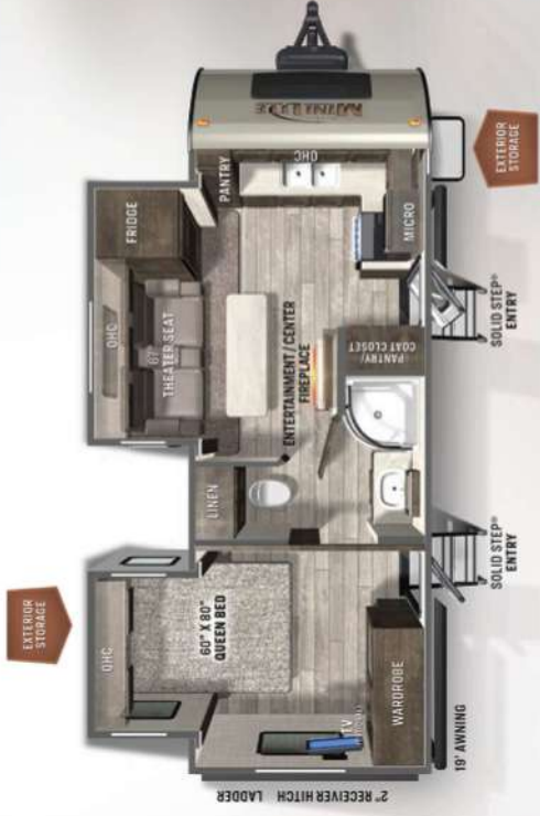
2516S FRONT KITCHEN MINI LITE UWW: 6033 HITCH: 810 AXLE: 5164 CCC: 1777 LENGTH: 25'11" WIDTH: 8' HEIGHT: 10'11" FRESH: 54 gal GRAY: 60 gal BLACK: 30 gal
