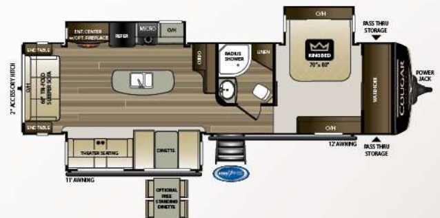
32RLI | Rear living room, three slides w/ bedroom slide Weight: 8416 LBS. | Length: 35' 11"
